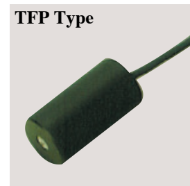
TFP Type For thin films. Inter-pin distance 1.0mm, pin points 0.15R, spring pressure 50g/pin. MCP-TFP
