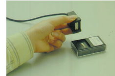
Use the probe checker to inspect probe connection.
